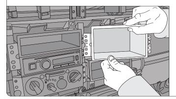
**Step 1:** Remove the dash panel, and then remove the two panels/compartment holders to the right of the radio.
