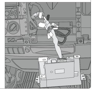
Step 2: Connect the end of the HRN-CI4A2 that is NOT marked OBDII to the FMS module.Next, connect the other end of the HRN-CI4A2 (marked OBDII) to the end of the HRN-CM24Y1 that is also marked OBD-II. See the third picture below.
