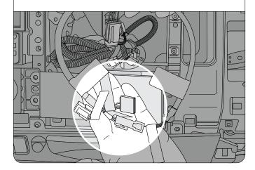
Step 3: Step 3: Once all harnesses have been connected, connect the GO9 device to the HRN-CM24Y1 and use the remaining cable length to mount the GO9 in a suitable location.
